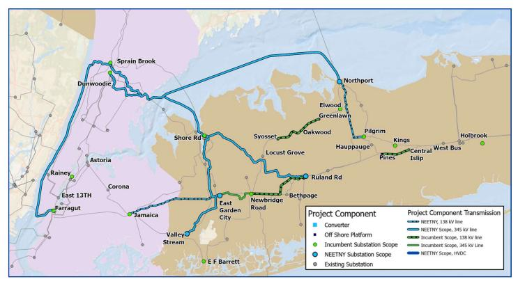
A highly cost-effective solution designed with geographic and electrical diversity to support flexible OSW injections, including from Eastern BOEM lease areas
