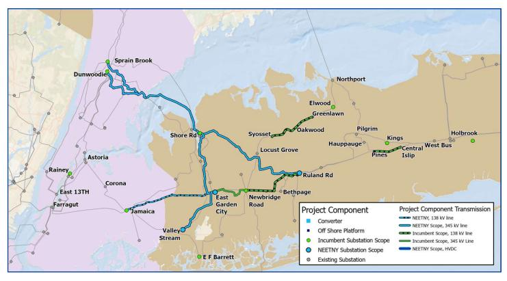
Builds upon Core 1, with an additional PAR controlled 345 kV tie-line between Zones J/K to increase operability and controllability
